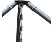
Attach the chain to the top Oring. So it'll be O-ring, carabiner, chain, carabiner, swing.
