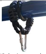
5. Connect the hanging ropes as above (wrapped over twice) and position it where you prefer. **This is important** to avoid wear from excessive rubbing.
