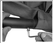
6. Tighten it with a bolt and washer
