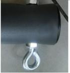
6. The eyelet bolt is inserted at the top of the C-curve, with eyelet pointing downwards, and should be attached **tightly**. Put a stick/screwdriver through the eyelet for leverage and tighten the nut with a spanner.
